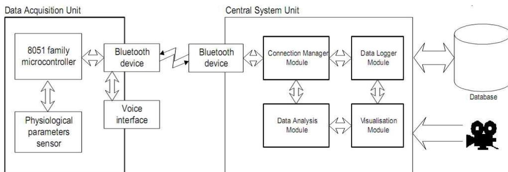
Figure.2 Block Diagram of System Design (Binyamin, 2010)
