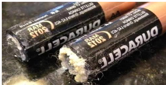
Figure1: leakage in chemical batteries
