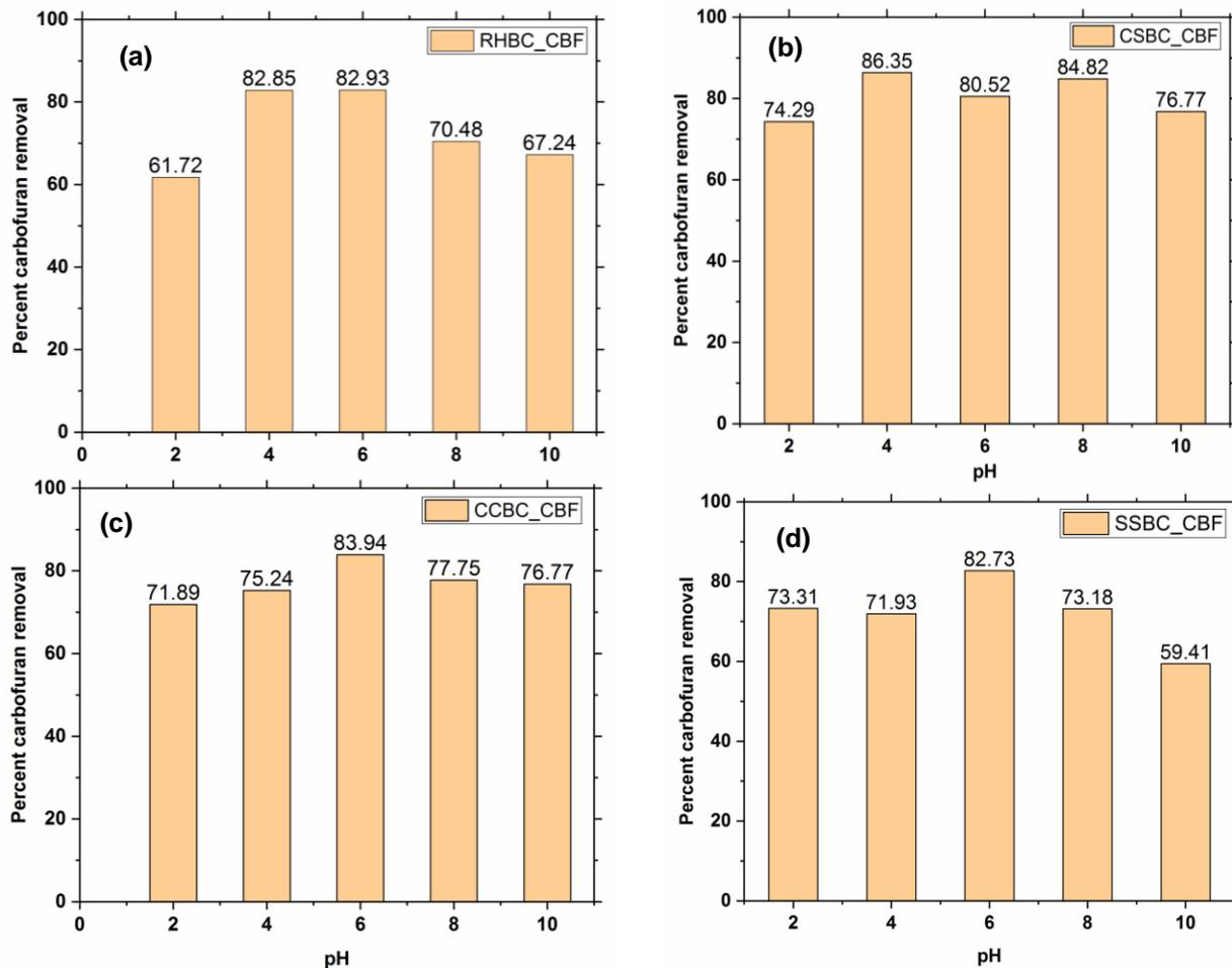
Figure 2: Percent carbofuran removal by (a) RHBC, (b) CSBC, (c) CCBC and (d) SSBC
