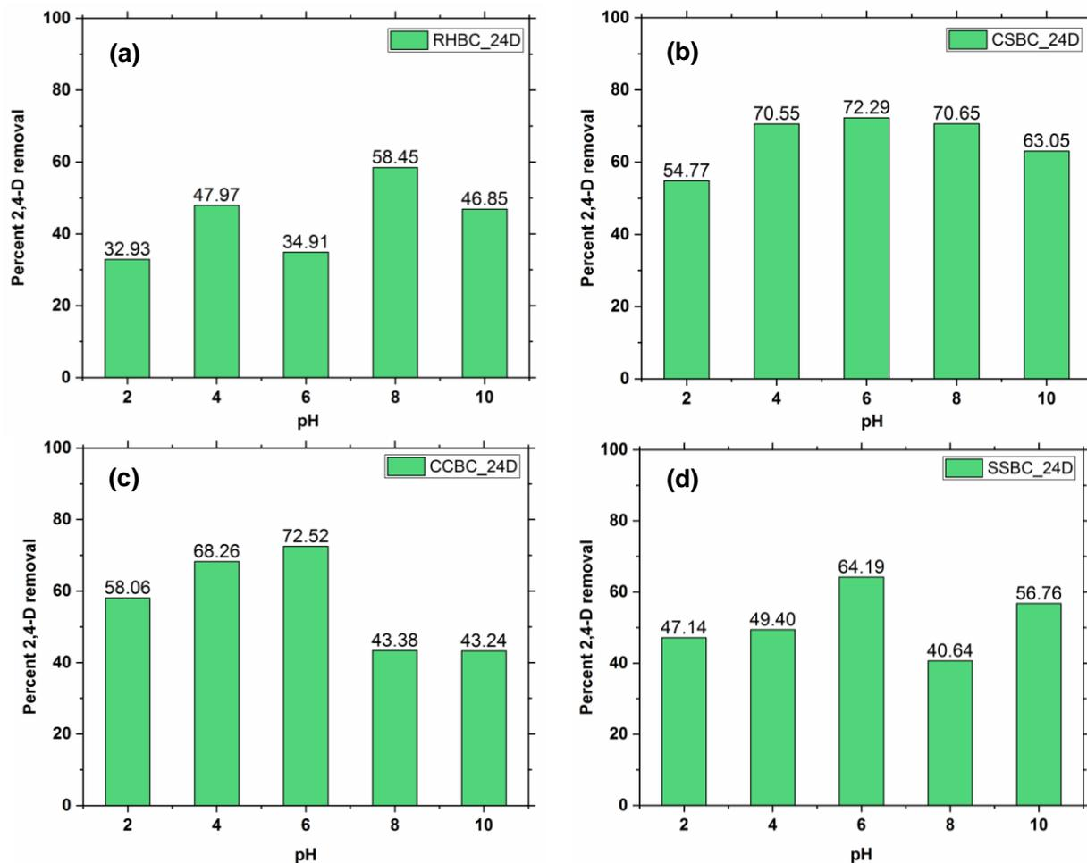
Figure 3: Percent 2,4-D removal by (a) RHBC, (b) CSBC, (c) CCBC and (d) SSBC
