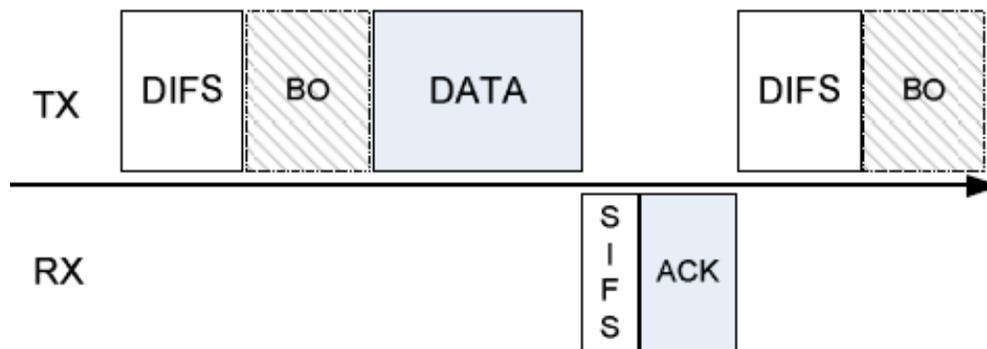
Figure-2.1 IEEE 802.11 DCF Basic Access Mechanism
