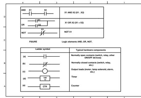
**Figure 2** Symbols for common logic and sequence components in a ladder logic diagram
