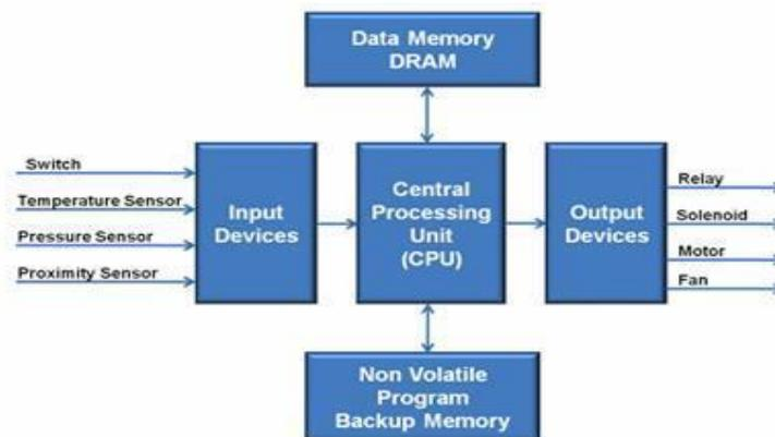
**Figure 3** General block diagram of the proposed PLC system
