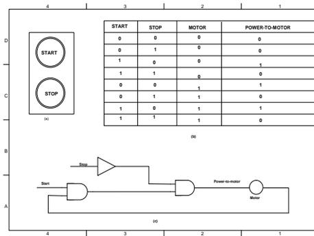
**Figure 1** (a) Pushbutton switch; (b) Its truth table; (c) Its logic network diagram
