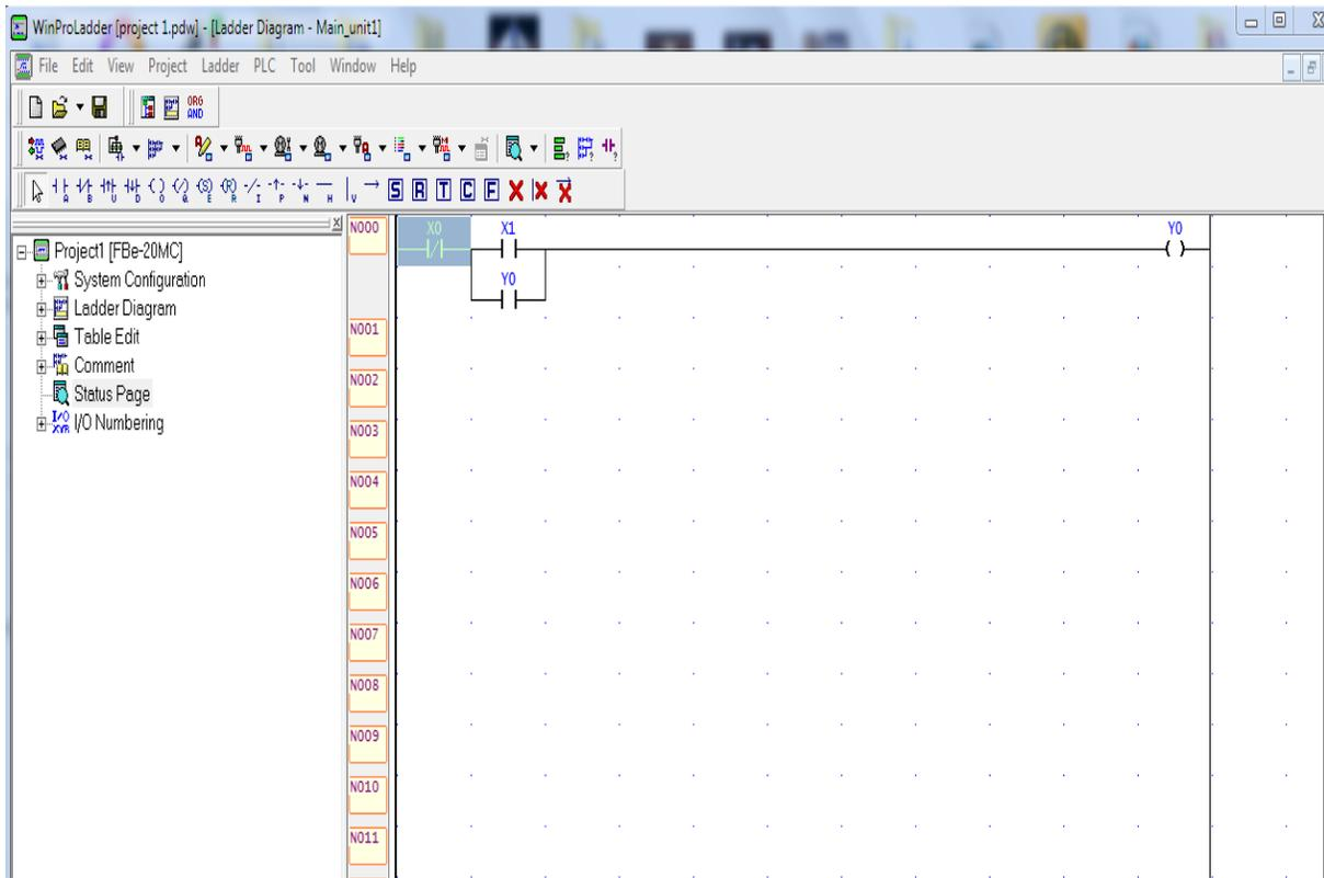
**Figure 9** Ladder Logic Program Window
