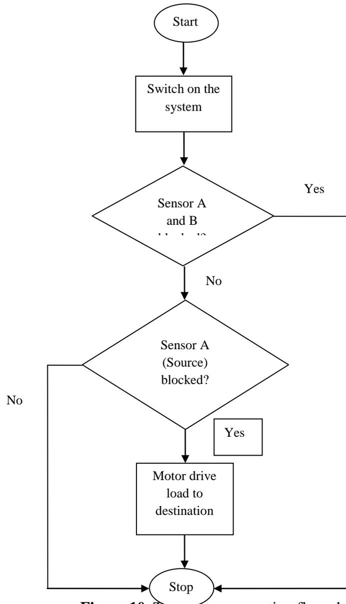
**Figure 10** The system operation flow chart
