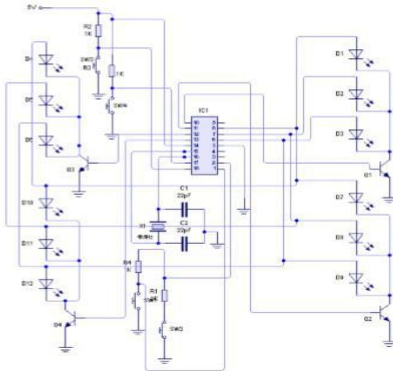
**Figure 3.0.** Circuit Diagram for Four Ways Emergency Based Traffic Light System
